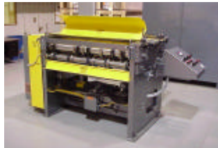
Upper & lower guards open for easy access to tooling
