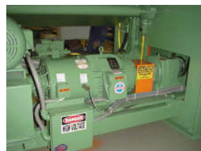
Totally self-contained drive & hydraulic unit
