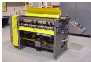
Upper & lower guards open for easy access to tooling
